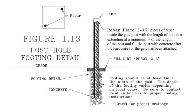
Prior to filling the posts with concrete it is important to screw the gate hardware on the gate posts so you are not screwing into a post filled with concrete. Gate hardware placement does not have to be exact and placement should look something similar to the gate specification diagram provided. At this point the gate hardware should be secured only to the post that will hold the gate up and not the gate itself.
