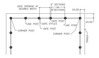
Once you have drawn the fence layout (sample above) and received your vinyl fence materials, it is time to mark the locations to dig the holes for the posts.
