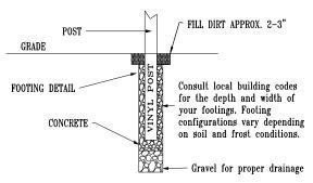
Safety Tip: When open holes exist, safety standards should be applied to properly protect the area and notify bystanders of the potential trip and fall hazards that exist with open holes in the ground. Clearly mark the area as a
