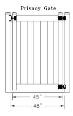
During the post installation process, there is no need to worry about the hardware or any other gate factors, simply focus on setting the gate post to the right spacing height, level and plumb. (See concrete mounting section if you are installing your post on concrete.)
