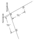
Important: If you have purchased 6' wide panels, the center to center measurement between any two posts should never exceed 6 feet. If you purchased 8' long panels, the measurement between two posts should never exceed 8'.
