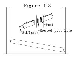
The rail can be secured to the post by using notches, rail clips, screws, or glue tabs. Notching is commonly used when a notching tool is available, when one is not available, glue tabs, screws, or rail clips are acceptable methods to secure the rail
