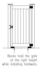
Secure the hinges to the gate with the provided screws and adjust the hinges to make sure the gaps on both sides of the gate are equal and the gate is level and swinging properly.
