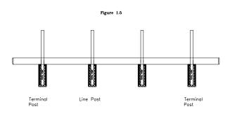
To set the post in a straight line you want to level the post and then place the post just off the string line (you do not want the post touching the string line).
