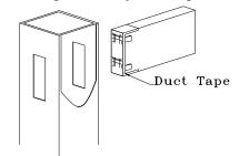
Once you have the right consistency, pour the concrete inside the post and fill the post with concrete. Typically installers use a cup or Gatorade bottle that has been cut at the top to form a funnel. Concrete will likely spill down the side of the post during this stage of the installation. Concrete can be wiped off easily if done before the concrete is allowed to cure. Typically we let the concrete dry a little on the outside of the post as we have found it wipes off easier
