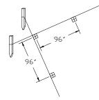
Important: If you have purchased 6' wide panels, the center to center measurement between any two posts should never exceed 6 feet. If you purchased 8' long panels, the measurement between two posts should never exceed 8'.
