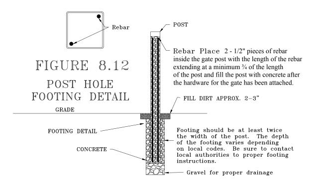
Prior to filling the posts with concrete it is important to screw the gate hardware on the gate posts so you are not screwing into a post filled with concrete. Gate hardware placement does not have to be exact and placement should look something similar to the gate specification diagram provided. At this point the gate hardware should be secured only to the post that will hold the gate up and not the gate itself. See Figure 8.13.
