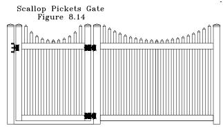
Attach the latch to the gate. The latch pin should fit loose into the latch.
