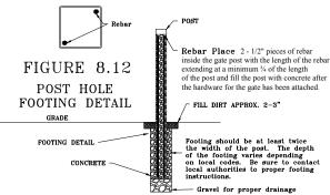
Prior to filling the posts with concrete it is important to screw the gate hardware on the gate posts so you are not screwing into a post filled with concrete. Gate hardware placement does not have to be exact and placement should look something similar to the gate specification diagram provided. At this point the gate hardware should be secured only to the post that will hold the gate in place and not the gate itself. (See Figure 8.13)
