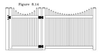
Secure the hinges to the gate with the provided screws and adjust the hinges to make sure the gaps on both sides of the gate are equal and the gate is level and swinging properly.
