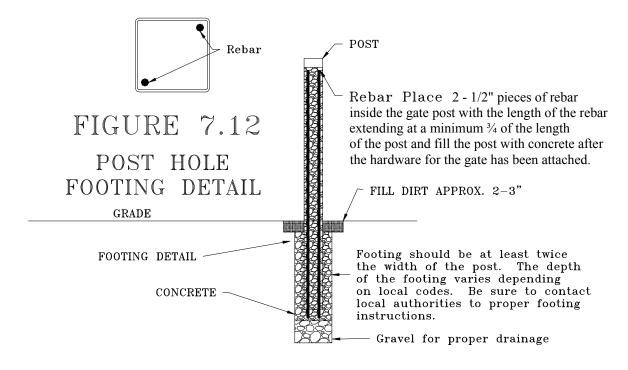
Prior to filling the posts with concrete it is important to screw the gate hardware on the gate posts so you are not screwing into a post filled with concrete. Gate hardware placement does not have to be exact and placement should look something similar to the gate specification diagram provided. At this point the gate hardware should be secured only to the post that will hold the gate up and not the gate itself. See Figure 7.13.
