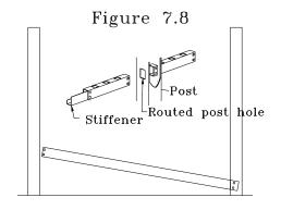
Note: When cutting a picket fence rail it is important to make sure that the distance from the first and last picket hole in the rail are equal in distance to each post. This process involves cutting both ends of the rail equally. See Figure 7.9.
