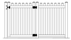
Secure the hinges to the gate with the provided screws and adjust the hinges to make sure the gaps on both sides of the gate are equal and the gate is level and swinging properly.
